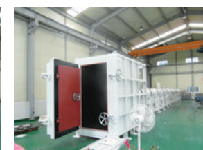
Explosion resistance Test Apparatus
